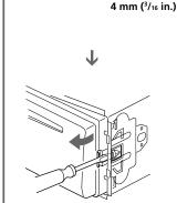
**2** Insert a flathead screwdriver between the
